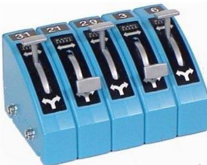
The Turnout Controllers are blue plastic electrical switches, with snap connectors on both sides (male on one, female on the other) which allow a row of controllers to be snapped together. The DC Controller is snapped to the left side of the first Controller to supply electricity to the entire row. A socket on the back mates with the plug on the cord from the turnout motor, or from the Turnout Extension Cord, where used.
