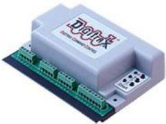
The Digitrax DS64 can operate four (4) 2-wire bi-polar solenoid turnouts (as well as other types), and the Kato 20-310 #6 Double Crossover. Each output can handle two turnout motors. Power can be track power or an external power supply such as the Digitrax PS14. As well as throttle control the DS64 can be controlled by push-button switches.
