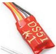
The Digitrax DS51K1 can be mounted under the T-TRAK module below the corresponding turnout. It is rated at 0.5 Amp and measures 0.319" x 0.509" x 0.152" (8.11mm x 12.94mm x 3.88mm).
